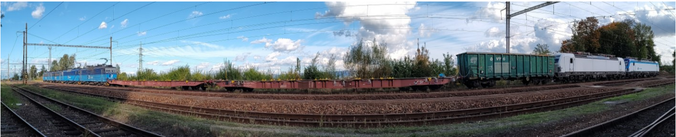
Fig. 7 Photography of the train set consisting of: 2x 193D + Eamnooss + Sggnss 80' + Sggnss 80' + 4x 363.5
